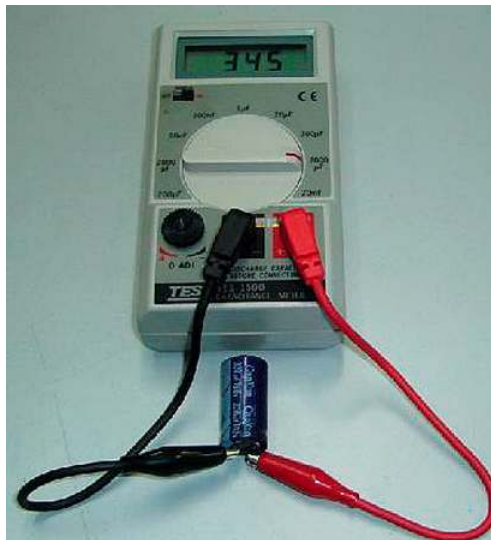
Testing capacitor with instrument intended for this purpose.
