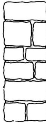
Bond stones or through stones provide stability to the masonry wall
