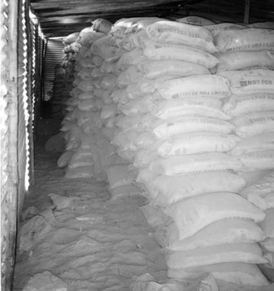
Improperly stored cement results in loss of quality
