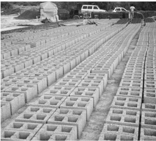
Concrete hollow block (CHB) production yard
