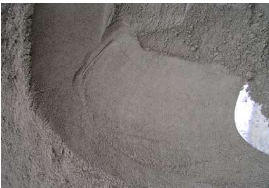
Flatten the dry mix with a trowel, if properly mixed a uniform gray color is visible.
