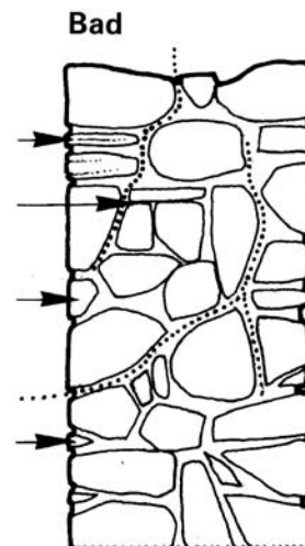
Bad example, stone wall construction with too many small stones and no proper bonds
