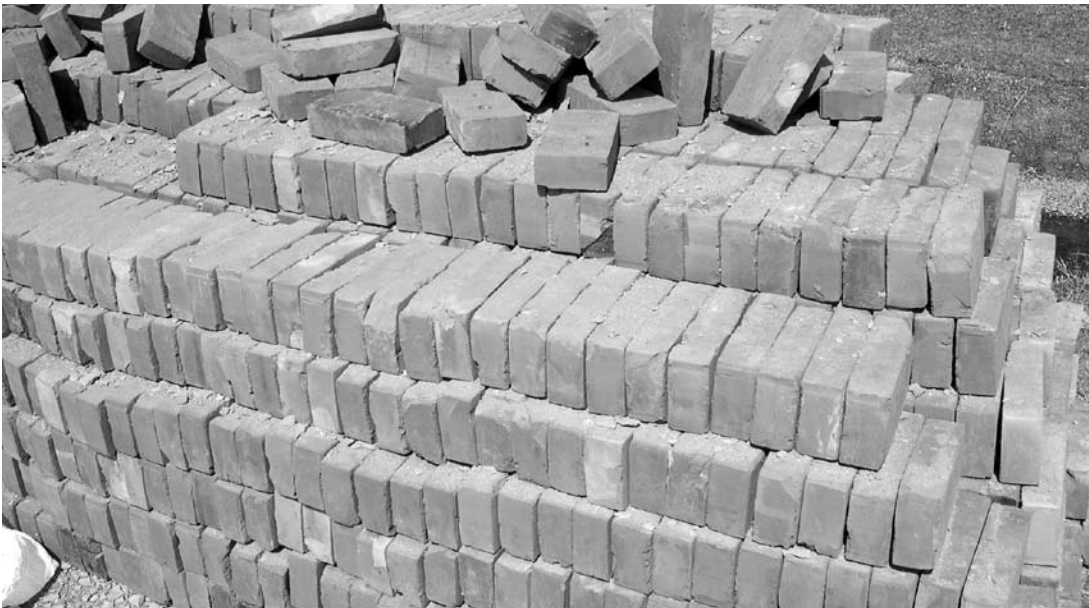
Facing bricks (second quality) stored at construction site
