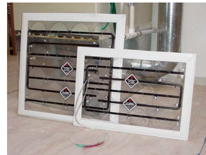
Figure 12. The Energy Conservatory TrueFlow flow grid.
