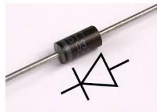
Representing anode and cathode of a practical diode through its symbol
