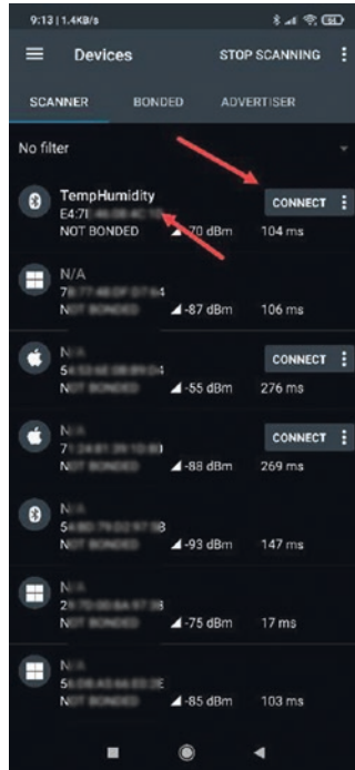
Figure 4-12. Detecting the TempHumidity BLE service
