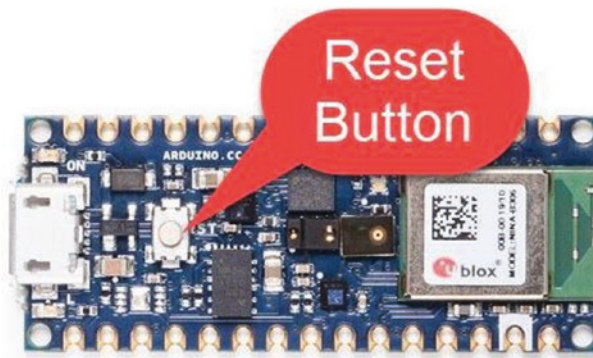
Figure 2-4. Position of the Reset button on the Arduino Nano 33 BLE Sense board
