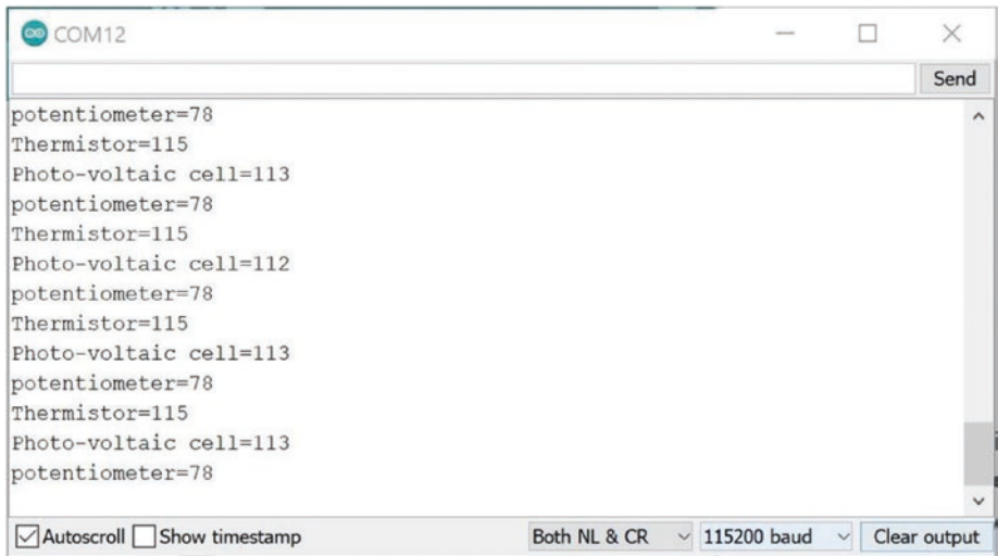
Figure 2-24. Program output for reading sensors over I2C
