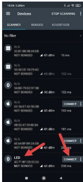
Figure 4-7. LED service shows in nRF Connect for Mobile application
