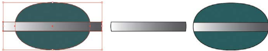
Figure 7.11 Two selected objects (left), intersect results (center), copy of original oval placed behind intersect results
