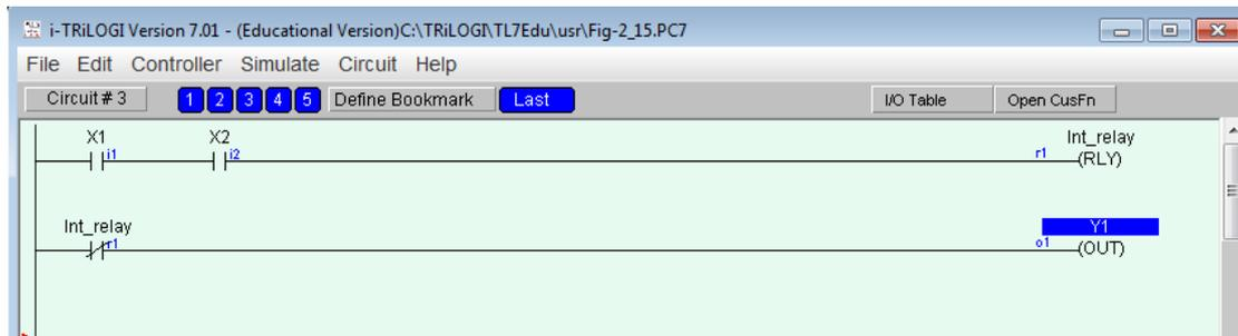
*Fig 2.15 Use of internal relay*
