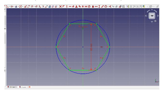
Close the sketch and then pad the sketch with 50 mm using the pad dialogue found on the tasks tab in the combo view window.
