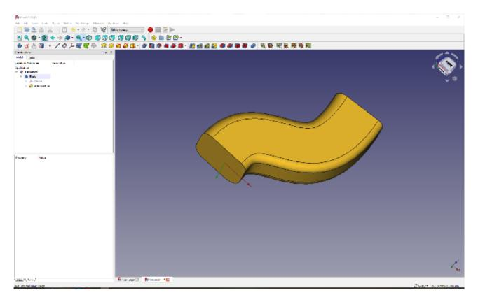
There are many other options in the sweep utility in the Part Design workbench that can change the way that corners are handled in a swept object, and also how it handles transforming from one profile to another profile over the course of a sweep, which you will explore on the part workbench shortly. The other thing of note on the Part Design workbench is that there is a blue and red icon that is the same as the sweep tool you used, except that it's for subtractive sweeps.
