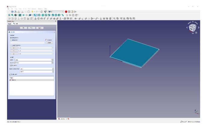
You could make this base part in a much easier way – namely, you could use the 'Create a cube solid' tool. However, as an example, you wanted one part to be made from an extrusion as you need to treat extruded parts a little differently when you get to the LCInterlocking workbench.
