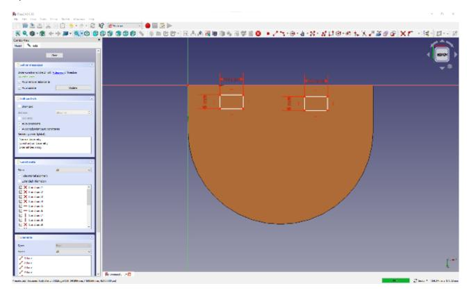
Then use the zero axis point to locate the closest rectangle to it, 8 mm across and 4 mm down from the straight edges of the design using the horizontal and vertical distance constraint tools and a corner point of the rectangle, as you have done with other items.
