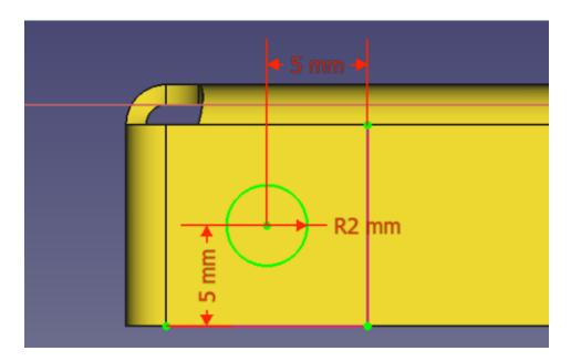
Closing the sketch, we then used the pocket tool on the Part Design workbench to create a hole, and selected 'through all' as the type so that the holes would be created on both sides of the design. Whilst we could have done this in a single sketch, we added another sketch to create the same holes at the other end of our tray.
