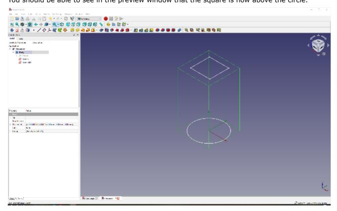
Next, making sure nothing is selected in the file tree, add a third sketch with this sketch drawn on the XZ plane. Using the 'create an edge linked to an external geometry' tool,
