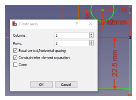
In the dialog, set the column and row number each to '2' and then tick the 'Equal vertical/horizontal spacing' checkbox as well as the 'Constrain inter-element separation' box. Clicking OK, if you now move your mouse around the sketch area, you will see a line protruding from your original circle; this represents the angle at which your array will be created and the distance from the original circle. Left-click to place the rectangular array of circles into the sketch.
