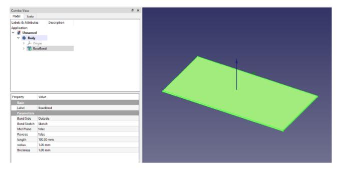
Next, let's select one of the edges on the BaseBend object. We selected the upmost edge line of one of the longer sides. With that selected, click the 'Extends one or more face, connected by a bend on existing sheet metal' tool icon, which should be second from the left in the Sheet Metal workbench toolbar.
