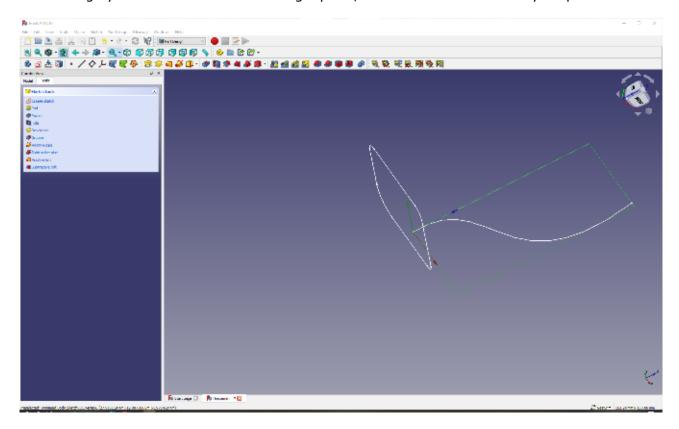
To sweep the profile along the curved path, highlight the first sketch you made and then click the yellow and red 'sweep a selected sketch along a path' tool.
