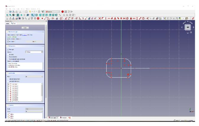
Close the sketch and then create a new empty sketch in the body. Create this new sketch in the XZ plane. In this sketch, you are going to create the path along which your first sketch profile will be swept. Let's use 'create a B-spline in the sketch' tool.
