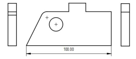
Adding the height of the 3D object is a similar task, except you don't have a single complete line from the bottom to the top of the object, so you will use vertices instead. Similar to the vertical and horizontal constraints in the Sketcher workbench, TechDraw can create a vertical dimension between two points, even if they don't sit on the same edge.
