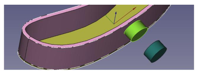
A common use for projection is to create 3D text effects. Let's first look at how to generate 3D text in FreeCAD, and then let's use some text and project it onto your curved surface again. Then you can combine projecting onto a curved surface with some Boolean part operations to create some interesting effects.
