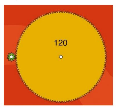
However, that 120-tooth gear will be physically quite large, and we might want to reduce the size. We could consider a 60:5 ratio, but, as a rule of thumb, gears with less than ten teeth begin to run not quite as well as their larger counterparts.
