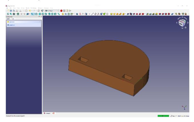
Next, cut slots that go into these pockets, so select the face of the back of the bird feeder object that need to be sketched on and create a new sketch.
