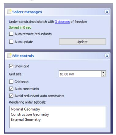
The aim is to reduce these degrees of freedom to zero by constraining all the items within a sketch. Constraining a sketch is the process of adding constraints that complete all the information about a sketch item's positions and dimensions. This is an incredibly useful
