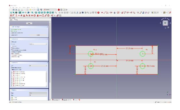
• L-bracket is 44 mm x 44 mm x 35 mm x 8 mm with holes of 6.2 mm located 10 mm from long side and 25 mm from short side while the pulley-hole is located in the middle at 8 mm from top
