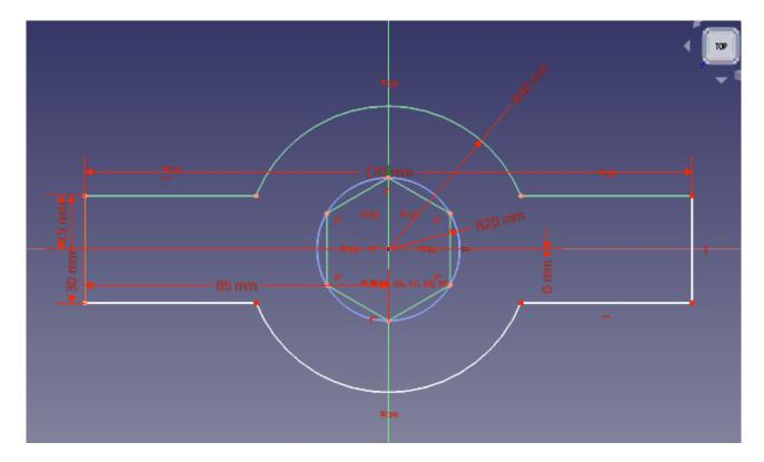
Moving back to the Sheet Metal workbench for a moment, we selected our sketch and clicked the 'Create a sheet metal wall from a sketch' tool icon again to create a basic BaseBend object.
