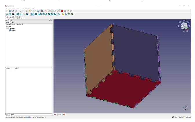
The next task is to apply the 'Export' tool to the tabbed parts you have generated. Rather than actually export a file, this tool explodes your box apart, lays the parts out as flat parts, and automatically creates a drawn shape projection of the parts. In the file tree, select all the new tabbed parts you created under the MultiJoin object, and then click the 'Export' tool icon.
