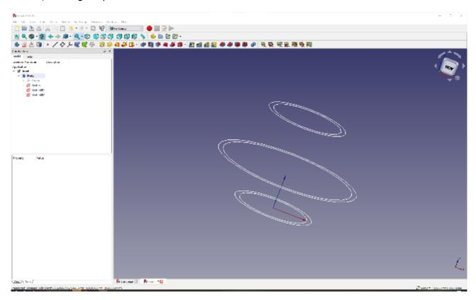
Create the loft in a similar way to the earlier example, starting by selecting the first sketch and then adding the second sketch and the third sketch in that order. If you uncheck the ruled option and the closed option, you should end up with a nice curvy shape.
