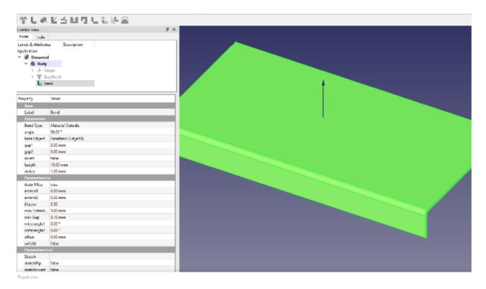
This new object appears in the file tree labelled 'Bend' and subsequent bends will be labelled 'Bend001', 'Bend002', etc.
