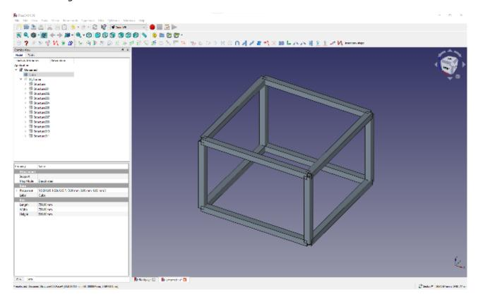
You'll notice that our frame has all the required sections but that they all overlap at the corners. We need to extend or trim these frame parts to make a frame that could be fabricated in real life. With the Open FrameBranch Manager still open, we can use the 'Get Targets' and 'Trim/Extend' buttons to help us do this quickly.
