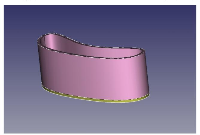
Previously, when you have worked with solid objects, you have often created sketches either attached directly to a flat face of an object or drawn on a plane, like XY or XZ, and then extruded or pocketed through an existing solid. With a curved object, such as the wall of your tray, drawing directly onto the surface is not really possible. However, you might often want to add design aspects to a curved surface. One approach to this is to use 'projection'.
