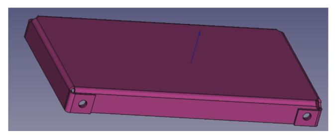
To fabricate an object, such as our tray created from a folded sheet, we need to be able to flatten our design back out after we have completed it.
