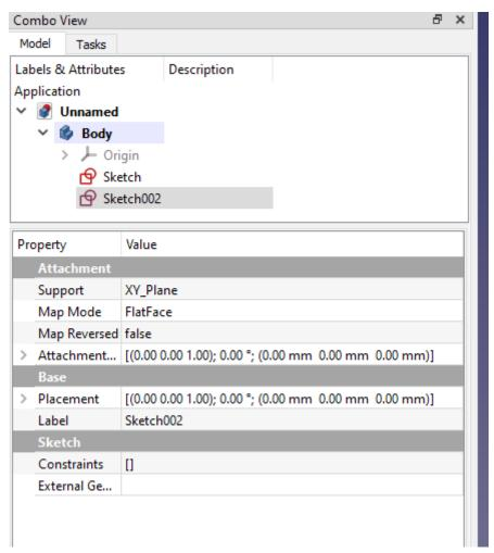
Making sure you are in the Attachment section, click the Attachment menu, and then click to expand the Position menu. In this drop-down menu, adjust the Z-axis to raise the hexagon sketch over the rectangle. This can be any amount, but I went for 20 mm. If you are in an isometric view in the Part Design workbench, you should see the hexagon sketch rise above the rectangle sketch.
