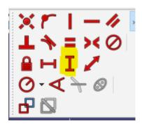
In the dialogue box that appears, type '20 mm', and then click OK. You should now see a red constraint label with '20 mm' in the viewer window – both vertical lines are now set to 20 mm. If you ever want to change this value, double-click on the constraint in the viewer window and the dialog box will reopen. You can click and drag the constraint around in the viewer window, and as you add more detail and constraints, you might do this to keep things clear.
