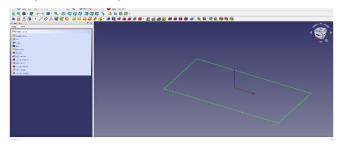
Without making further changes to this sketch, we can move straight away to the Sheet Metal workbench. In this workbench, with our sketch highlighted in the file tree, let's click the 'Create a sheet metal wall from a sketch' tool icon.
