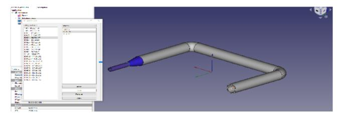
Finally, click the Insert button to insert the tube. Similarly, we can add a curved section or 'elbow' into the design using the 'Insert a Curve' tool.
