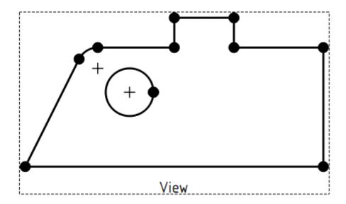
You'll notice that all the lines in the drawing have the vertices marked as dots (similar to the Sketcher layout). The vertices help us to add dimensions and other tasks, but they are part of the view frame. You can toggle the view frames on and off by clicking the 'Turn View Frames On/Off' icon, or by right-clicking and selecting 'Toggle Frames'.
