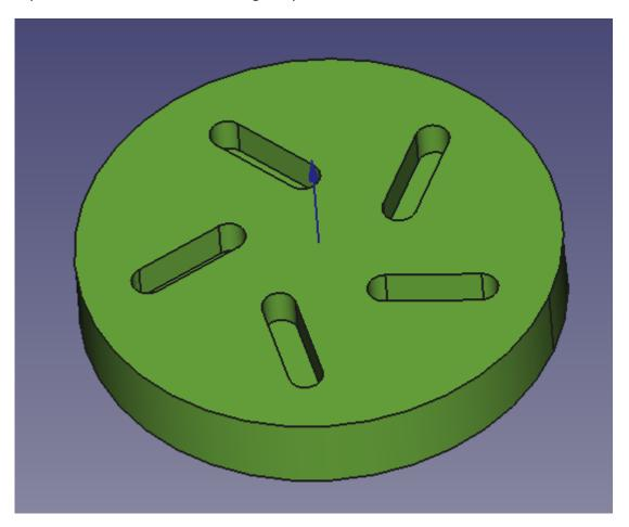
You can of course go all the way back to the root sketch of the pocket and adjustments will be recomputed to the pattern array. Close the polar pattern dialog and open the slot sketch in the file tree. In the slot sketch, constrain the slot so that the centre of the slot is positioned on the Y axis datum line.
