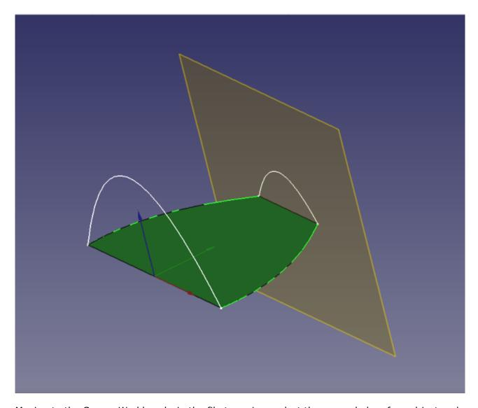
Moving to the Curves Workbench, in the file tree view, select the new ruled surface object and select the two sketches that create the rear and front edge shape of your canopy design. With these three objects highlighted, click the 'Sweep profiles on 2 rails' tool.
