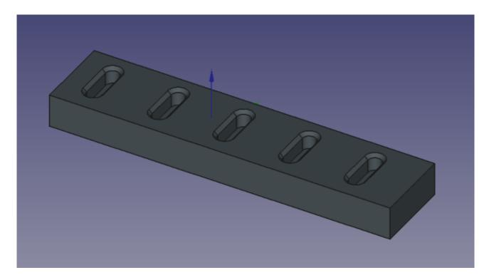
Removing a feature is slightly counter-intuitive in that you can't select the feature to remove in the list in the 'Add/remove feature' box in the dialog. Similar to adding a feature, you click the 'Remove feature' button and then highlight the feature in the preview or in the file tree view.
