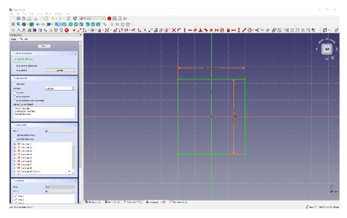
Close the sketch and perform a 'pad' task to extrude the box; set the pad dimension to receive the input from the box height cell, B3, in the spreadsheet. Next, you will click the upper surface of your box and use the thickness tool you explored earlier to hollow out your box. To set the thickness, you are going to link the thickness value in your spreadsheet, B4. you make it an outwards thickness. All being well, you should now have a hollow box in the preview window.
