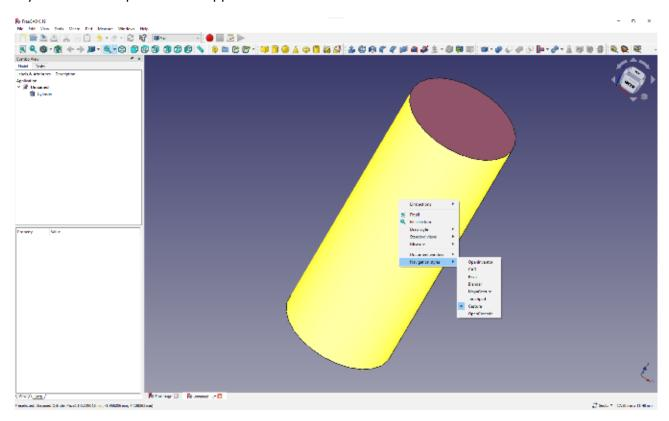
Some of the navigational styles are based on other CAD environments, so if you are used to using, for example, Blender, then you might prefer that style. You use the 'gesture' style option that gives left-click for rotation in the document window, right-click for moving, and the centre button/wheel is for zooming. Of course, you need an object like the cylinder you created to allow you to judge which navigational style suits you best.
