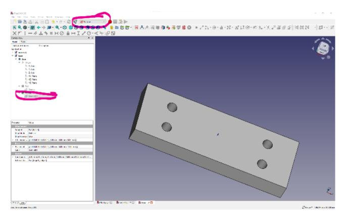
Close the sketch and then save the base part project by clicking the Save button. Now close that project tab. Notice that the base in your partly assembled project hasn't changed. To update the parts, click the 'Update parts, which have been imported to the assembly' tool icon (a yellow part icon with two curved green arrows over it).
