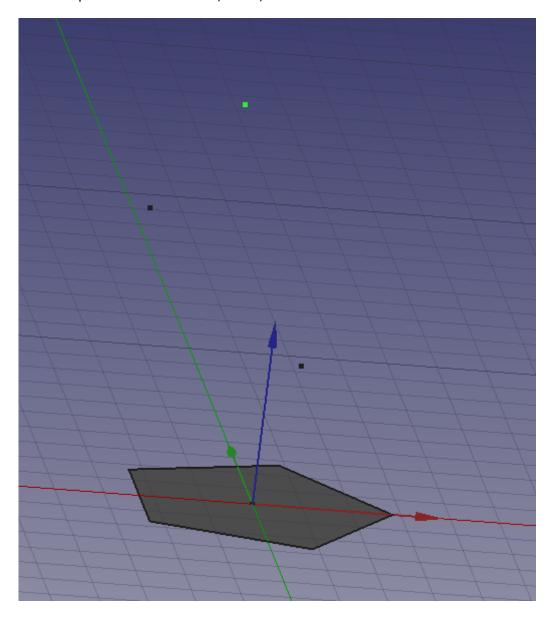
Creating a curve between the points you just made is easy with the 'Create a multiple-point B-spline' tool.
