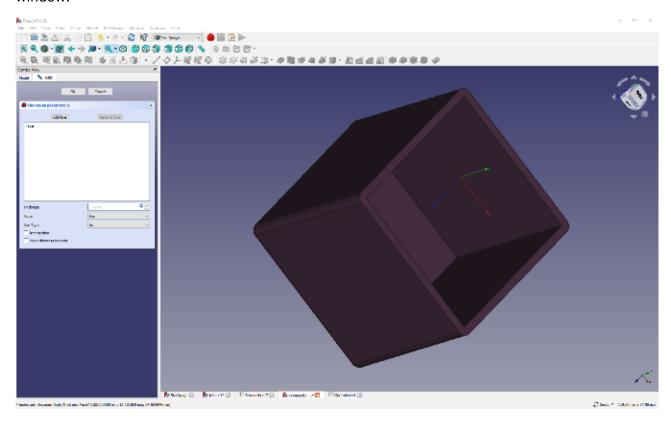
To make a lid, you are going to do the same process as you did to make the box section, but you are going to use some simple formulae so that the lid is generated to fit whatever dimensions are of the box created.
