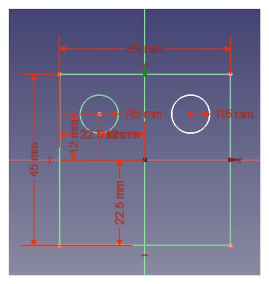
Of course, you can then select the two circles and the X axis datum line and repeat the process to create two more circles in the lower left and right corners.
