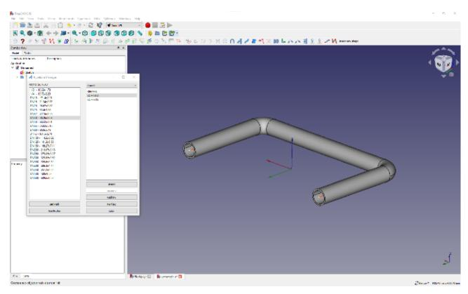
We mentioned earlier that you can add pipe objects and other peripherals by simply attaching them to an existing pipe. There are numerous tools that help us do this. Selecting the outer edge of one end of our U-bend pipe construction, click the 'Insert a Reduction' tool.
