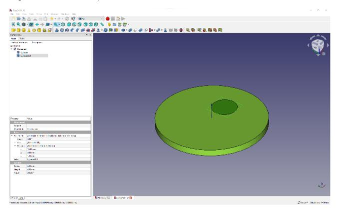
The next operation is to subtract the second smaller cylinder out of your first to leave a 2 mm deep pocket. To do this, hold the CTRL key down whilst selecting both the cylinders in the file tree. Next, find the 'Make a cut of two shapes' tool . Click the button, and the smaller cylinder should be cut out of the larger disc.
