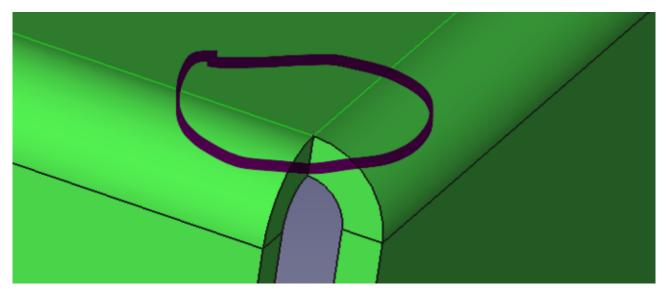
With the two lines selected, the 'Corner Relief to sheet metal corner' tool icon should become active.
