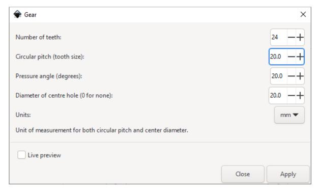
First, check that the Units option is set to 'mm', then you can experiment with 'Number of teeth' and the size of the tool using 'Circular pitch (tooth size)'. The pop-up also neatly has an option to include a hole in the centre of the gear, as you'll often want to mount it on some kind of shaft. We'll talk about the 'pressure' or 'contact' angle elsewhere in this chapter, but for now it's a good idea to leave it set to the default 20 degrees.
