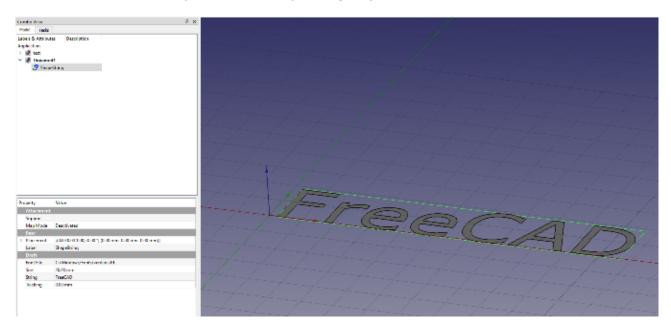
Now that you have a ShapeString object, you can move back to the Part Workbench and perform the usual sort of operations upon it. Whilst not totally necessary, if you extrude the ShapeString on the Part Workbench a little, say 3 mm, it means that you can use the simple 'Transform' operation you used earlier to move the object into your projection position.
