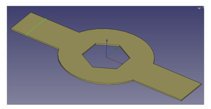
To create this fold, you first need to select the face where the sketch is attached on the BaseBend object in the preview window. This feels a little counter-intuitive and we naturally would select the whole BaseBend object in the file tree, but this doesn't work. With the correct face selected, hold the CTRL-key and click the sketch in the file tree. With these two items highlighted, you should now see that the 'Fold a wall of metal sheet' tool becomes visible.
