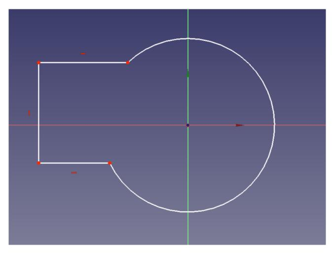
If we now try and use the 'Trim and edge with respect to the picked position' tool, we will get an error message. The Trim tool is only of use when a line intersects or is connected to another line.
