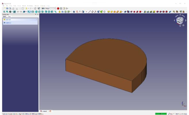
For the rest of this project, you are going to create more sketches, but these sketches are going to be drawn onto faces of the pad object you have just made. The first job is to make a pocket for the bird feed to be contained in. So, left-click in the viewer to select the upper face of the object.
