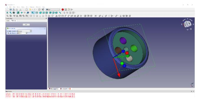
As you made a 'simple copy', your new wheel doesn't contain the hierarchy of operations and objects your original has and also is not dynamically linked to the original object. This means that if you make further changes to your original 'wheel', these aren't pushed through to the simple copies. However, of course, you can delete the copies, make a change to the design, and recopy if needed.
