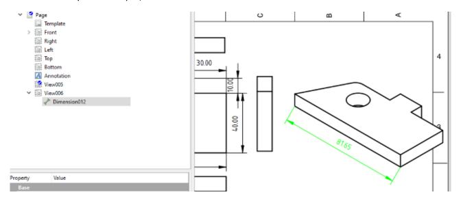
Having noted that, click over to the 3D object tab and highlight the same edge on the 3D object. Next, click the yellow 'Link Dimension to 3D Geometry' tool.
