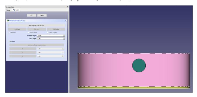
click the 'Project edges, wires, or faces of one object onto a face of another object' tool.
