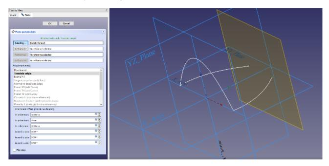
With the new datum plane highlighted in the file tree, click the 'Create a new sketch' tool to open a new sketch. Import the B-spline endpoints to the sketch and make a smaller B-spline to form the front of the canopy in the same way that you did the sketch for the canopy rear on the XY plane.
