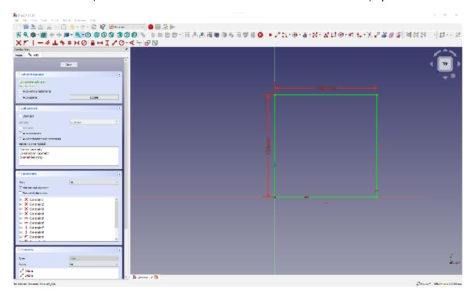
Having drawn the square sketch, use the 'extrude/pad' tool on the Part workbench to extrude the sketch to a thickness of 3 mm. Using 3 mm means you can imagine you are going to laser-cut your tabbed box out of 3 mm plastic or plywood.
