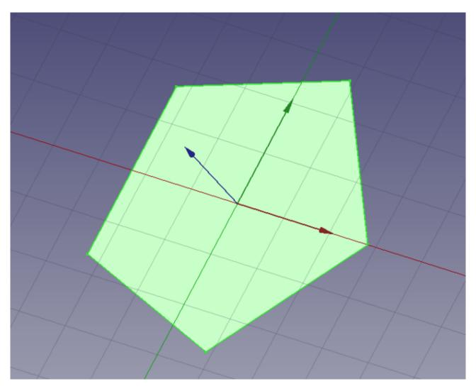
Next, let's create some points which you will use to create a curved line in three axes. The first point of the line is going to be the centre of your polygon, or the zero point. Click the 'Create a point object' and click to place a point at the datum.
