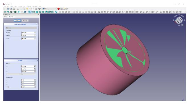
Next, perform a cut to remove the new cylinder from the design. You then continued to make the wheel look a little fancier by creating four more cylinders of 2 by 12mm. You moved the four cylinders equally outwards by 5 mm from the centre of the wheel using the moving techniques you learnt earlier. You should end up with a simple wheel.
