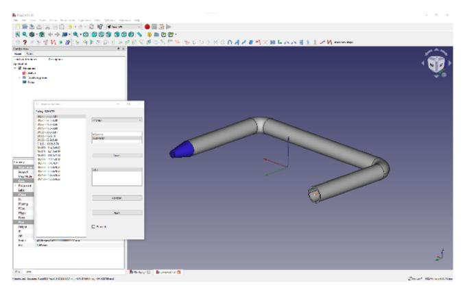
It's as straightforward to add a simple length of straight pipe to an existing design. Again, select the edge of the thin end of the reduction we just added and click the 'Insert a Tube' tool.
