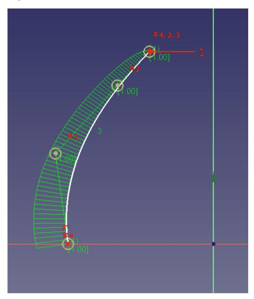
Before you close the sketch, select the B-spline that you just made and click the 'Create a symmetric geometry with respect to the last selected line or point' tool to add a mirrored B-spline on the right-hand side of the Y axis line.
