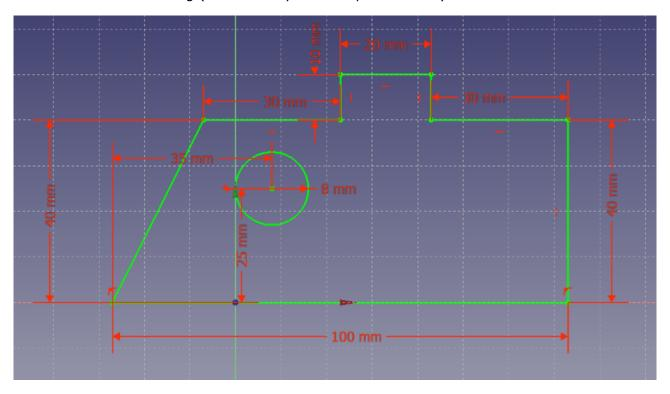
Having drawn the outline, add a circle in the object, and then close the sketch and perform a pad operation of 10 mm on the sketch to create your part. Finally, before you jump into the TechDraw workbench, add a fillet to an external edge with a 7 mm radius.
