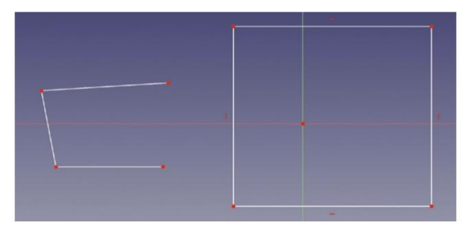
Next, select the 'Extend an edge with respect to the picked position' tool and left-click on one of the lines that doesn't meet the rectangle. If you move the cursor, you can now extend this line to any position you like or, as it crosses the line forming part of the rectangle, that line will become highlighted meaning that you can attach the line to the rectangle at that point.
