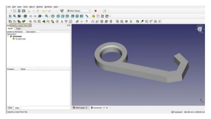
The Mesh workbench has some tools that are similar in approach to the Part workbench, where you create simple solid objects and combine them using Boolean functions to stick objects together, or subtract one shape out of another. If you want to turn around the hook part of your mesh file, you will create a copy of the hooked end and rotate it using these tools.
