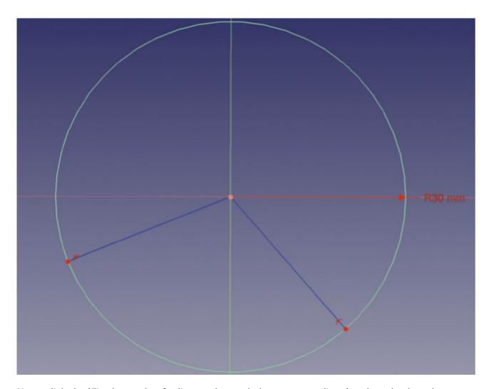
Next, click the 'Fix the angle of a line or the angle between two lines' tool, and select the vertical Y axis line and then the lower right-hand construction line.
