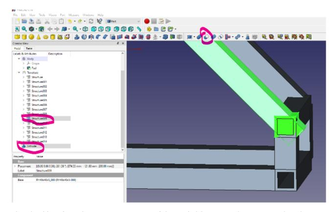
This should perform the correct cut on one of the angled frame members. Next, select the other frame member you wish to cut excess material from and then select our extrusion object, which now can be found inside the 'Cut' object folder that was just created in the file tree.
