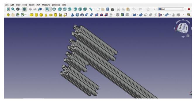
One way you could make this easier is to draw an aluminium extrusion profile sketch, and then pad or extrude it multiple times to multiple lengths. As a workflow, you might choose to use the Part Design workbench to create a body for your original extrusion and then create multiple simple copies on the part workbench.
