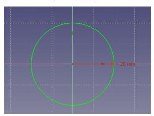
Having constrained the sketch, you now pad it to 50 mm, make an inner tichnes of 3 mm and remove the bottom.
