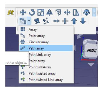
This applies an array without a pop-up dialog box, but the resulting array has some editable parameters in the Combo View window. You should see the array has been created with four instances of the smaller cylinder placed equidistantly around the larger cylinder edge. If you highlight the array object in the file tree and adjust the 'Count' parameter, it will add or remove instances from the array and redistribute the count to maintain equal distances between each instance.
