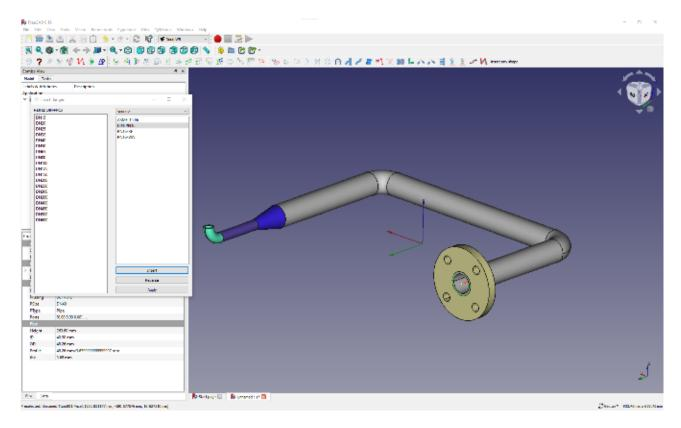
We're sure by now that you have the general idea, but it's worth exploring the other tools available to manipulate and create pipe systems. There are tools for adding valves of differing types, U bolts to secure pipes to other structures, tools to cap the end of pipes, and tools to create flowing branches in pipes. There really isn't much you can imagine that you couldn't design using these tools.
