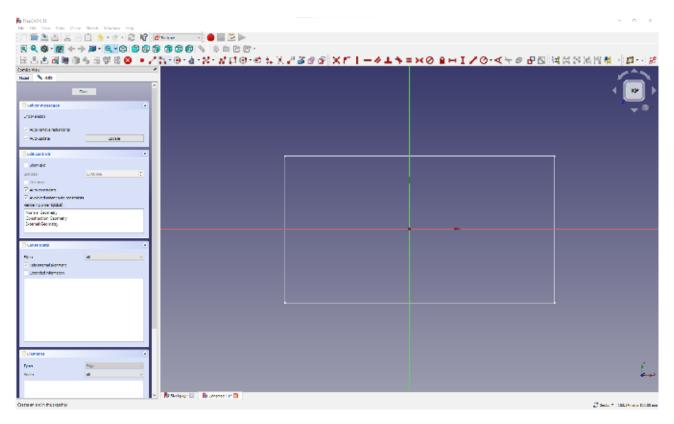
In the Part Design workbench again, within the same body, create a second sketch. Click the 'Create sketch' button, and select the XY plane for your second sketch. In this second sketch, use the regular polygon tool to draw a hexagon that is smaller than the rectangle you drew – draw it inside the rectangle, and don't worry if it overlaps a little. Again, you don't need to constrain the hexagon, so close the sketch.
