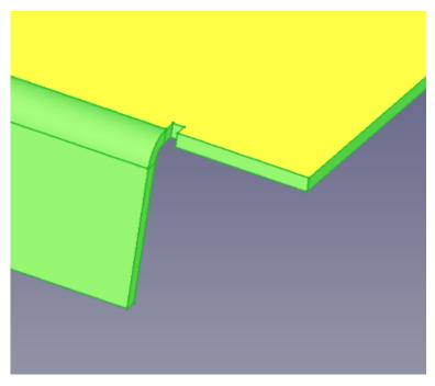
If you wanted to not have a relief notch added, you can scroll down to the 'Parameters relief' section and set the relief factor to '0' and then set the 'use relief factor' setting to 'true'. This option might be useful if you are using the Sheet Metal workbench to design using different materials, such as thin card or plastics.
