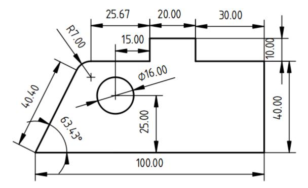
Slightly differently than the Sketcher workbench, when you want to select multiple vertices, you need to hold the CTRL key down. Select the right-hand vertex on the bottom edge of your object and the highest vertex on the right of the small bit that sticks up at the top of the design. Click the 'Insert Vertical Dimension' tool to add the dimension and note that it correctly adds the vertical distance between the points – not the distance along a straight line between the points.
