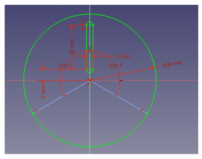
Select the 'Create a slot in the sketch' tool, and make sure you have toggled the drawing tools back to normal mode and you aren't still drawing in construction mode.
