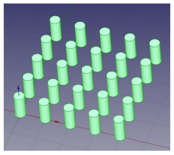
Highlight the array item in the file tree and delete it. You should now see your cylinder item and if you highlight it and press the SPACE bar, we'll make it visible again. Next, let's try the 'Polar array' tool from the Array tools drop-down menu.
