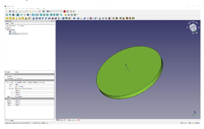
You are now going to repeat the above process to make another cylinder; this should appear in the file tree as 'cylinder001'. Change the size of this cylinder to a radius of 6 mm and a height of 2 mm. It will now appear to have disappeared, as it is underneath your original cylinder. In the dialog box, expand the 'placement' drop-down and then the 'position' drop-down, and let's change the position of this cylinder. Change the z coordinate to 1.3 mm. This raises the
