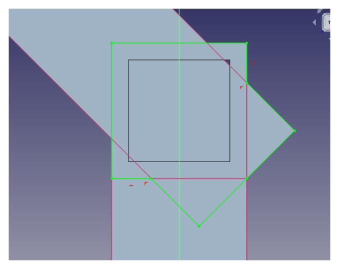
Next, close the sketch and move to the 'Part' workbench and extrude the sketch you just created. Extrude it in such a way that it moves through the frame element you wish to cut material from. For me that is -40 mm.
