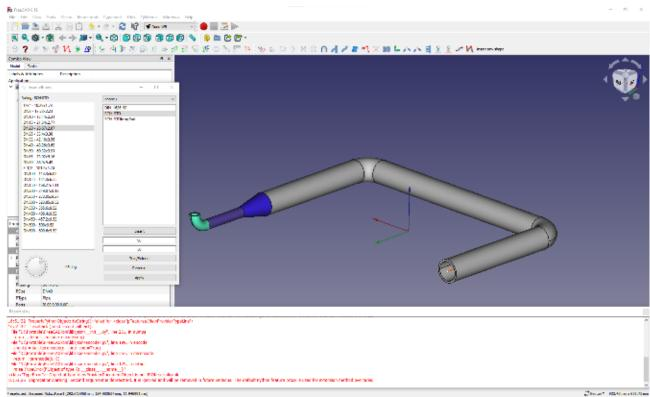
Often pipework uses flanges as joining mechanisms between pipe sections, and as such, the 'Dodo' workbench has a 'Flange' tool. At the other end of our pipe experiment, we selected the outer edge of the pipe end and clicked the 'Insert a Flange' tool.
