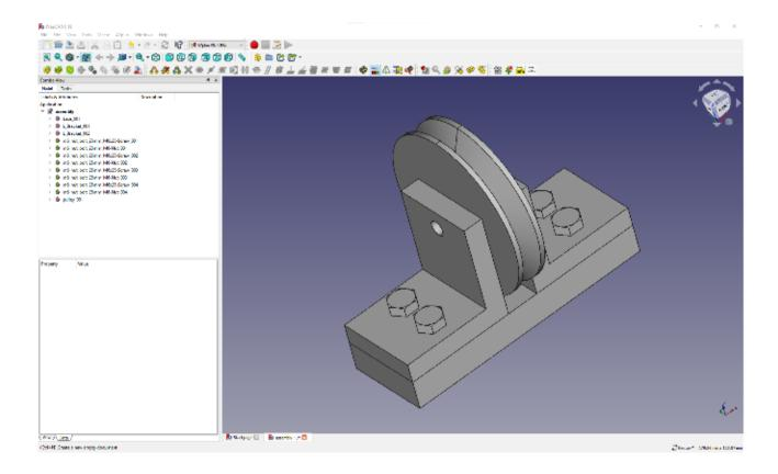
To finish your assembly, import the spindle bolt file and constrain it through the centre of the brackets and the pulley, then fit the nut to the other end. You are sure by this point that you can work out how to constrain this one into position without instruction.
