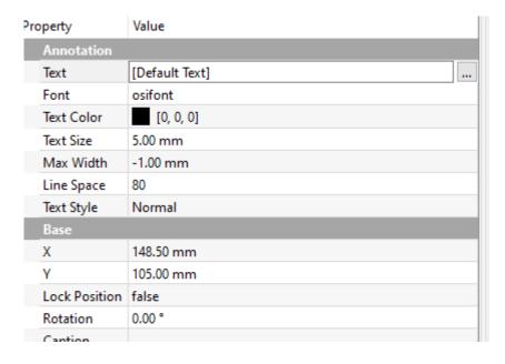
Note that it doesn't use text wrapping, and you need to hit your keyboard Enter-key to create a new line of text. In the image above, you have filled in the default drawing details with the editable text boxes, but also added some text in an annotation box outside the default drawing text boxes, as you can add an annotation frame anywhere in the drawing.
