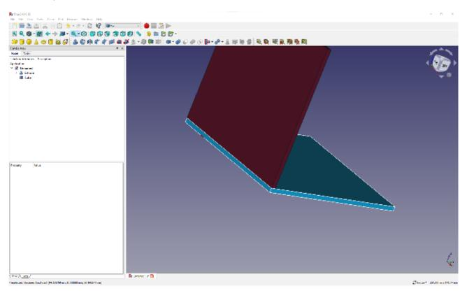
Make the opposite side of your box by either repeating the process and moving it to the opposite side, or simply copy and paste and move a duplicate of the first side.
