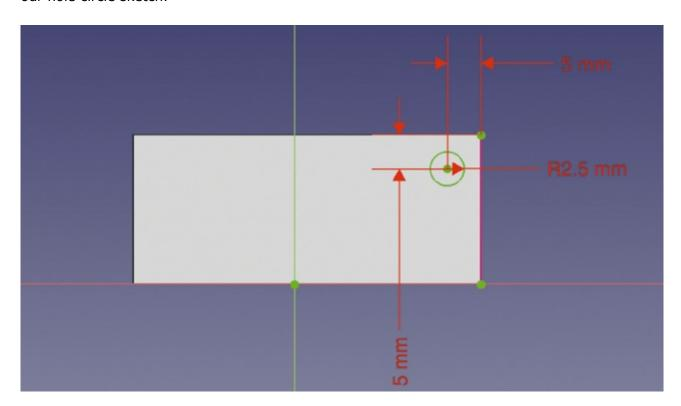
In essence, what we have done in our hole, in a cuboid example, is use an underlying geometry to create a guide point in the new sketch onto which we can attach constraints. We can see, therefore, that guide points can be incredibly useful, but often we may need a guide point in a position where there is no underlying geometry that we can import. An incredibly powerful feature of the Sketcher workbench is that we can switch all the drawing tools to 'construction' mode.
