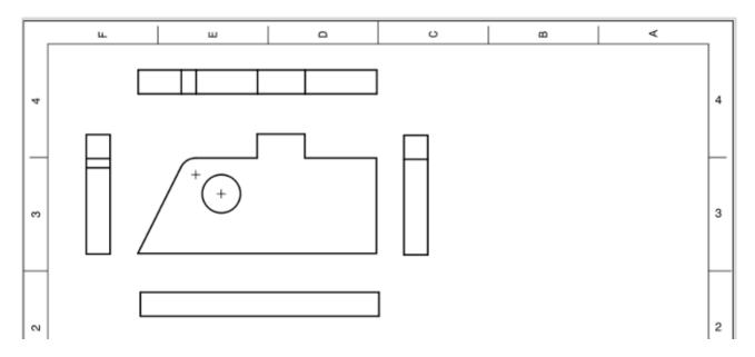
Next, let's add some dimensions to parts of the views so that someone could make this part accurately. It's similar in feel to adding constraints in the Sketcher workbench. First, let's select the long line/edge at the base of your object in the front view on the technical drawing page. Then click the yellow 'Insert Horizontal Dimension' tool icon.
