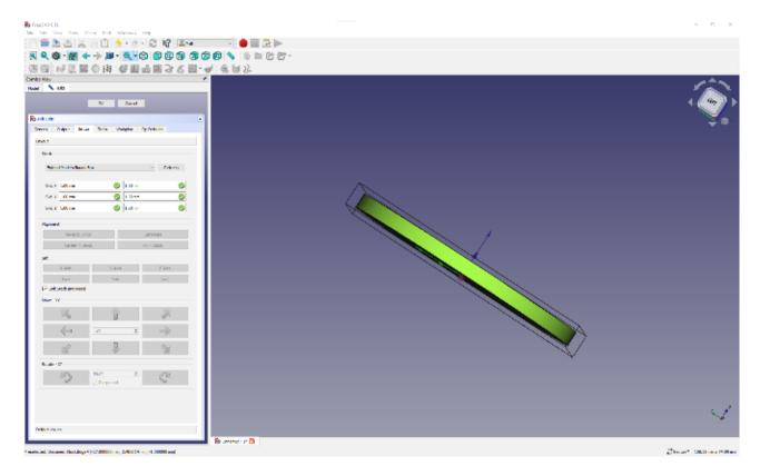
As you are going to use 3.13 mm plywood that is the correct thickness, you don't need any material above the surface of the disc. Therefore, you will adjust the z axis dimension of the bounding box in the 'Setup' dialog box to reduce the stock dimension to zero by changing the 1.00 mm on the second Ext. Z axis column to 0.00 mm.
