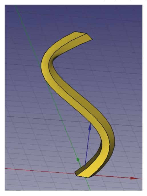
Moving back to the Draft Workbench, select the swept object in the file tree and then click the polar array tool icon. You put your centre of rotation at around  $-30 \, \text{mm}$  on the X axis to create your array of five of your swept items.
