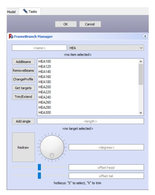
To create a frame, we need to select a profile for the frame extrusions. There's a collection of preset profiles included that model real-world standard metal extrusions. Let's select a simple  $40 \text{ mm} \times 40 \text{ mm}$  square extrusion with a 5 mm wall thickness. Click the drop-down menu that currently reads 'IPE' or 'HEA' and select 'RH', and then select the 'RH40×40×5' by highlighting it in the list below. Make sure to give it a name Eq: 'MyFrame'
