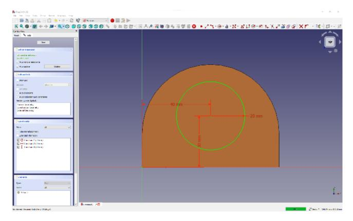
Close the sketch, and with this new sketch highlighted in the file tree, click 'Pocket' from the list on the 'Tasks' tab. You should now see that it's cutting the circle as a pocket into the bird feeder design. Eet the depth of the pocket to 8 mm.
