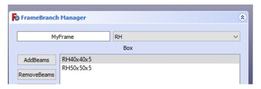
Next, click on any edge of the cube in the preview window and then click 'OK' in the Open FrameBranch Manager dialog box. You should now see that every edge of the cube object has had the  $40 \text{ mm} \times 40 \text{ mm}$  extrusion added to create a frame.
