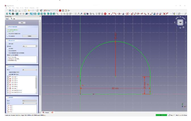
This sketch is the main outline of the bird feeder, so click 'close' on the sketch solver panel in the combo view window, and return to the Part design workbench. Make sure that the sketch you drew is highlighted in the file tree, then click the 'Tasks' tab just above the file tree view.
