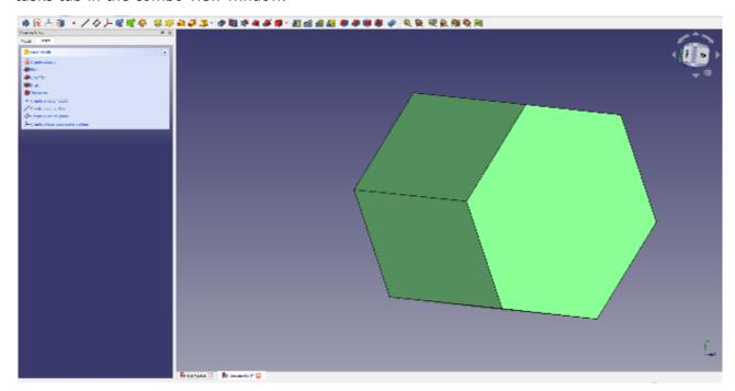
You are going to now use the thickness tool to hollow out your hexagonal extrusion. Select the upper face of the hexagonal extrusion and then click the 'Thickness' tool. You should see instantly that the part now appears as a hollowed version of itself. Make is 2 mm. In the thickness tool dialog, you can see the selected face and change various parameters
