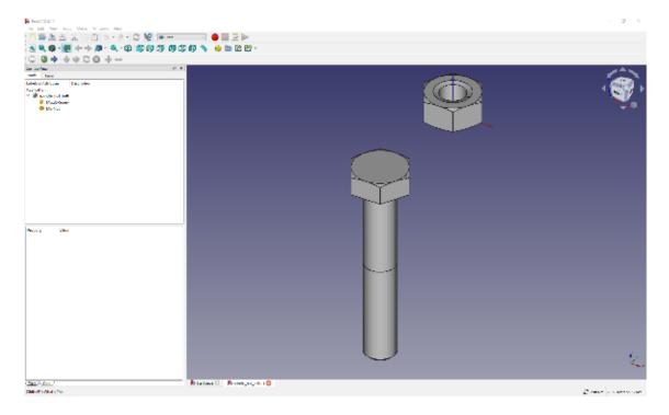
Now that you have all the parts, create a new project for the assembly in FreeCAD. For ease, save this new project in the same folder as all the component files.
