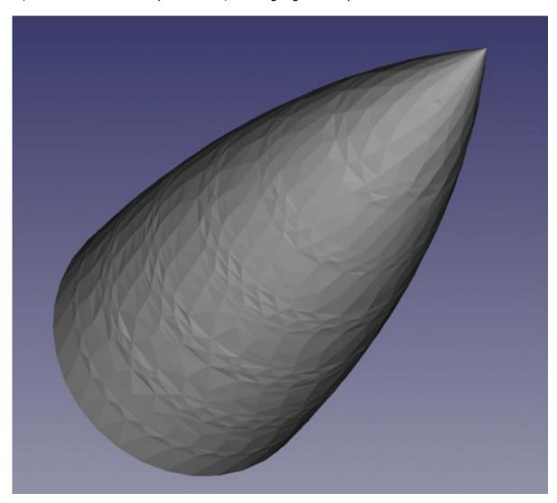
For this mesh, let's set the surface deviation to 0.03 mm and the angular deviation to 10 degrees. You should see that the resulting mesh is a higher resolution and more precisely matches the original part.
