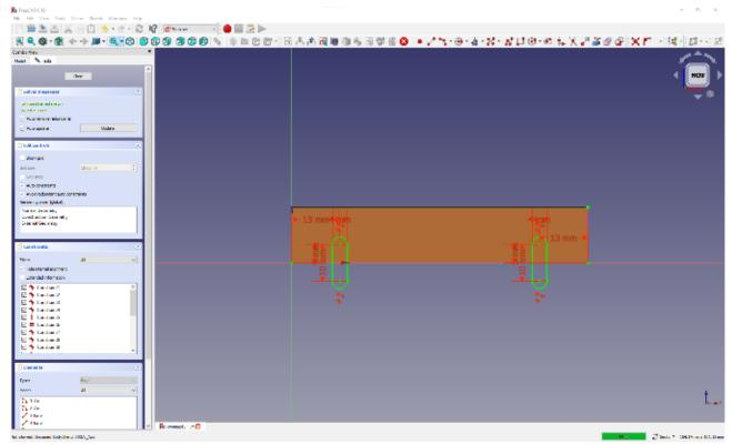
Close the sketch and again performed a pocket, setting the depth to 5 mm, to cut into the rectangular pocket, but not deeper into the object.
