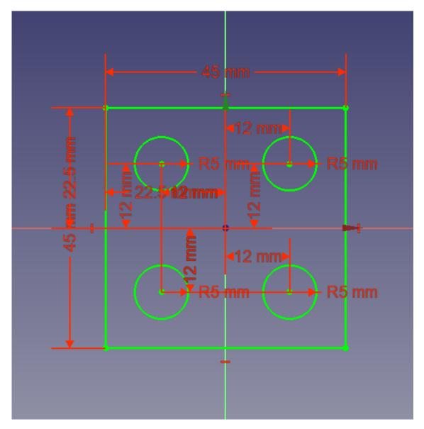
To create this sketch, you drew four separate circles and constrained each of them dimensionally and positionally. It's a fine approach, but it's quicker to use some of the cloning and array tools the Sketcher Workbench offers. In Sketcher these tools can create matching objects and carry over some of, or manipulate, the existing constraints to save us some time.
