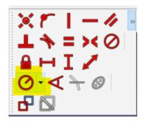
and in the dialog box, set the radius to 40 mm. You should now have a fully constrained sketch, with all lines turned green.
