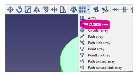
In the dialog, leave the polar angle set to 360 degrees to create a full circle array and set the number of elements to 5. You need to add a point which is the centre of rotation; if you left the centre of rotation set at the 0,0,0 point, you would simply create five cylinders placed on top of each other. Change the Y co-ordinate to 10 mm and then click the OK button. You should now see a circular array of five cylinders appear.
