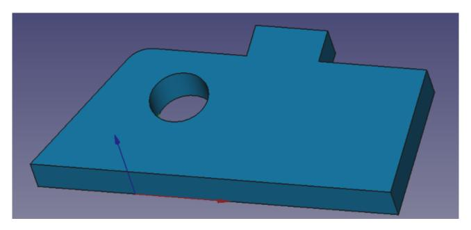
Having an internal hole and an external radius and an angled edge gives us enough details to do a good demonstration of the TechDraw workbench tools.
