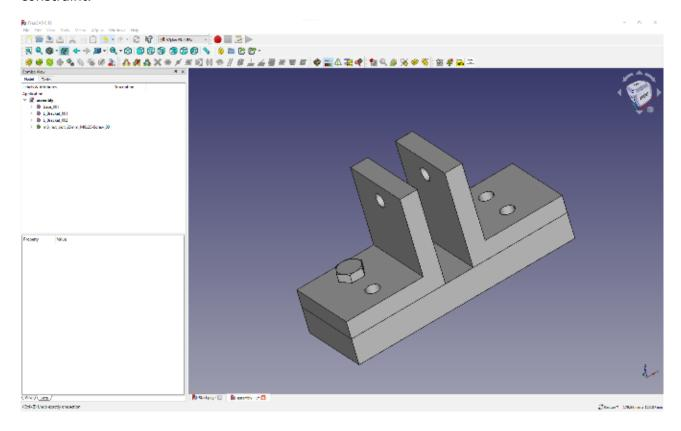
Moving to the nut, if you move the nut closer to the bolt end under the base, you can then select the edge at the base of the bolt before the slight chamfer and the lower similar edge just inside the nut. Again, apply a 'circularEdge' constraint to fit the nut to the bolt.
