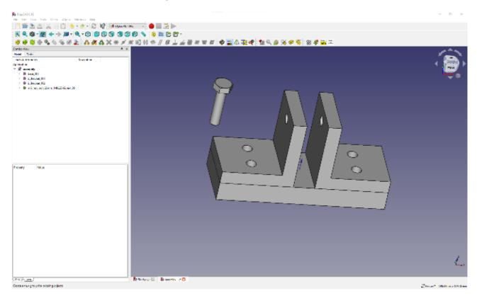
Let's constrain the bolt section first. Select one of the circle edges at the opposite end of the bolt from the head. Using the CTRL key, select one of the upper edges of one of the holes on the bracket. You want these two circles to align on an axis, but you don't want to constrain the edges together as the bolt end circle obviously needs to be out of the other end of the hole. Clicking the 'Add an axis constraint between two parts' achieves this – the bolt should now align to the hole.
