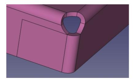
However, this piece currently sits inside/on top of the other folded wall section. Of course, this would be impossible to make, so we need to use an offset to place this fold correctly.
