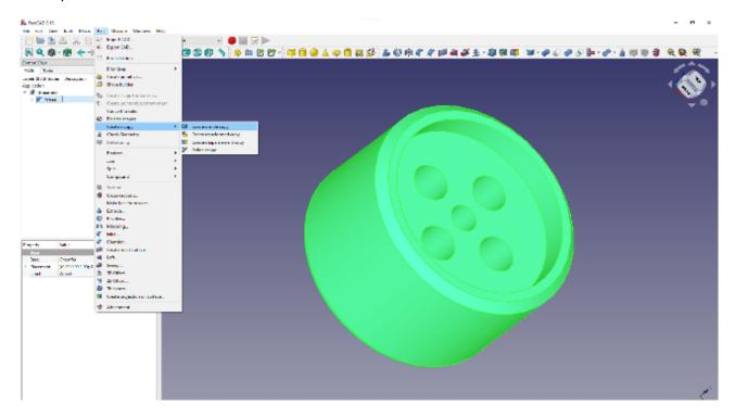
Clicking this option will create a new 'wheel001'. If you double-click on wheel001, you can see that it can now be moved in the 3 axises as well as rotate as a separate item. The behaviour of the change you can set in the 'Tasks' tab.
