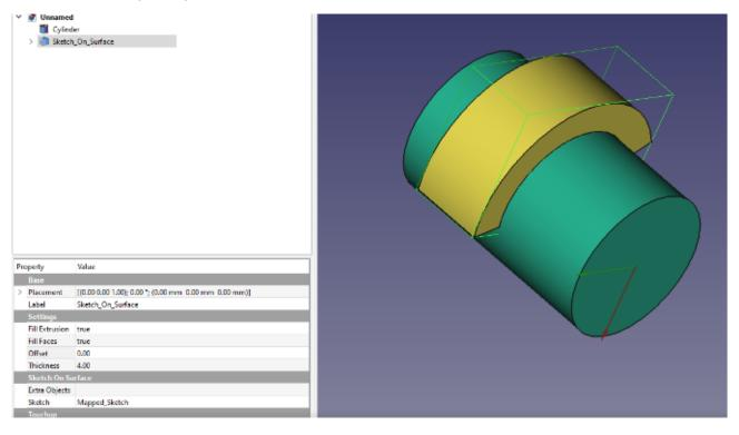
It's perhaps worth pointing out that the resulting objects made using mapped sketches work in the same way as other objects with regard to the Part Workbench and other tools. You can add some fillets to the edges of the part and use the appearance menu to set the object's colour. You can also go one step further in that you have clicked the surface of your mapped object and created another SketchOnSurface object to create the small extruded hexagon.
