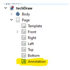
To edit the annotation, select it in the file tree view. In the combo view, you should now see the editable parameters of the annotation, which include common text editing options like font and size. At the top of the annotation parameters, you should see 'Text' and the 'Default Text' that is stored within it. Click the ellipsis icon (the three dots to the right) and in the pop-up window you can input text.
