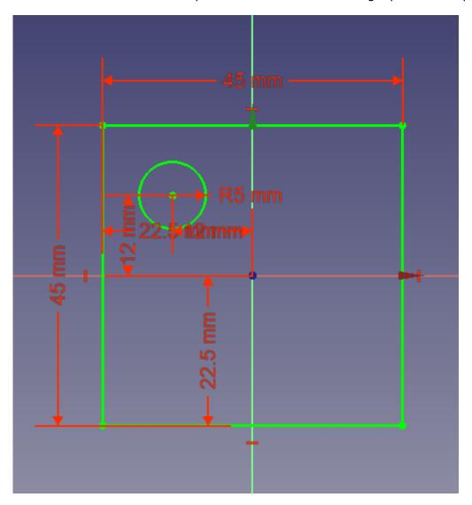
Next, select the circle and the Y axis datum line. You can now click the 'Create symmetric geometry with respect to the last selected line or point' tool icon.
