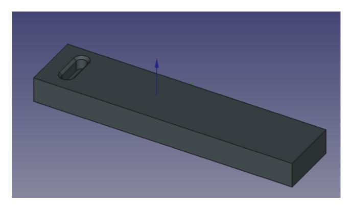
The Part Design Workbench has some specific array tools, and you are going to try the 'Create a linear pattern feature'. With nothing selected in the file tree, click the linear pattern tool.
