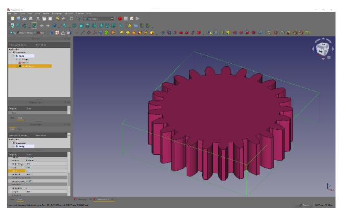
We have made a 25-tooth gear that is 7 mm tall. Notice that we have created this inside an active body that we set up on the Part Design workbench.
