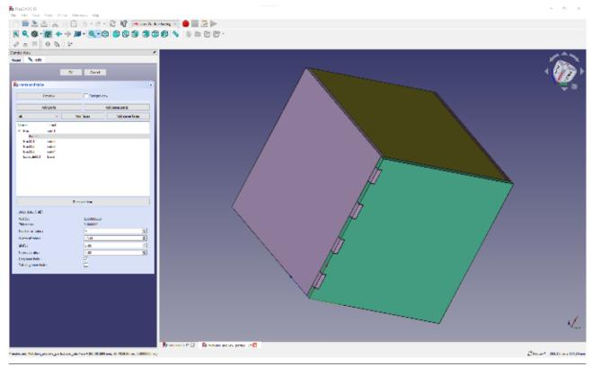
You can now repeat the above process of selecting and adding faces to the interlocking dialog and configuring tabs. Working your way through the model, you added tabs to the other three faces that interlock with the base, and then added tabs to two of the side panels to create tabbed joints on every interface of your box.
