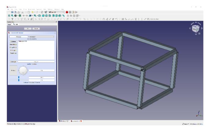
It's worth noting that although we have used a solid object as the basis of our frame, we can apply frame structures directly to sketches. As a quick example, create a new project and move to the 'Part Designer' workbench and create a sketch that has a rectangle with an extra line spanning across the rectangle inside – our rectangle was  $1000~\text{mm} \times 500~\text{mm}$ , in the XY-plane. Note that you might need to click 'Fits the whole content on the screen' to view the retangle.
