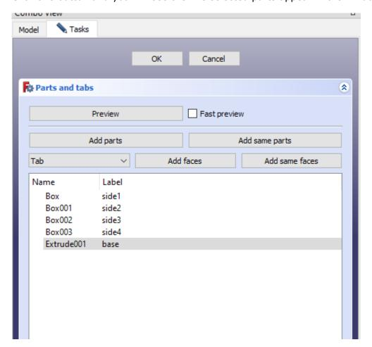
This list of parts in the dialog box is similar to the file tree in the combo view in that you can highlight anything in the list – you can press the SPACE bar to toggle visibility. This is very handy for the next task. You need to tell the 'Interlocking' tool which faces of your box are going to interlock. Let's begin with the faces that will form the tabs that extend into the base. Select the 'Base' part and then press the SPACE bar to make it disappear – do this for three of the sides.
