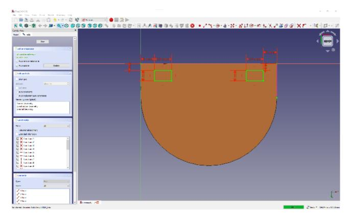
Having constrained the rectangles sketch, close the sketch and performed another pocket operation to a depth of 10 mm.
